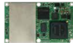
Advanced BD970 OEM receiver designed for various applications.
