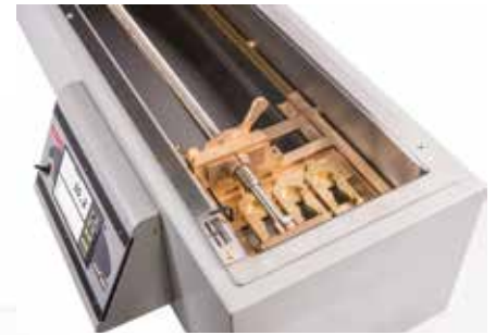
Interior of HA-1068 showing test molds, screw drive and disengage lever.
