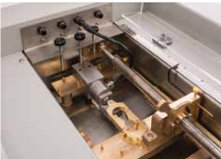
Interior of HA-1060 showing HA-1066 force determination transducer set up.
